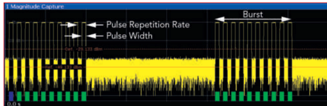
Fig. 2 The burst signal consists of 10 pulses followed by a pause.
