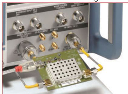
▲ Fig. 1 The R&S FSWP phase noise analyzer feeds a pulsed signal to an amplifier, then analyzes the amplifier's output.
